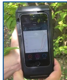
Fig 3. The Biomeme two3™ thermocycler displaying qPCR results.
